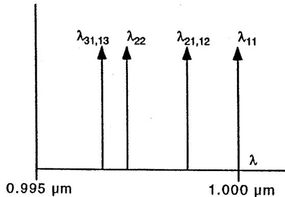
Figure 1.16. Mode spectrum including first six lateral modes.
