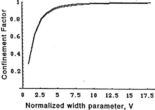
Figure 1.17. Confinement factor vs. V as waveguide width is varied.
